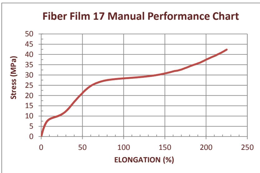
The graph above illustrates how the film performs under an increased load. Where the line ends indicates where the film breaks.
